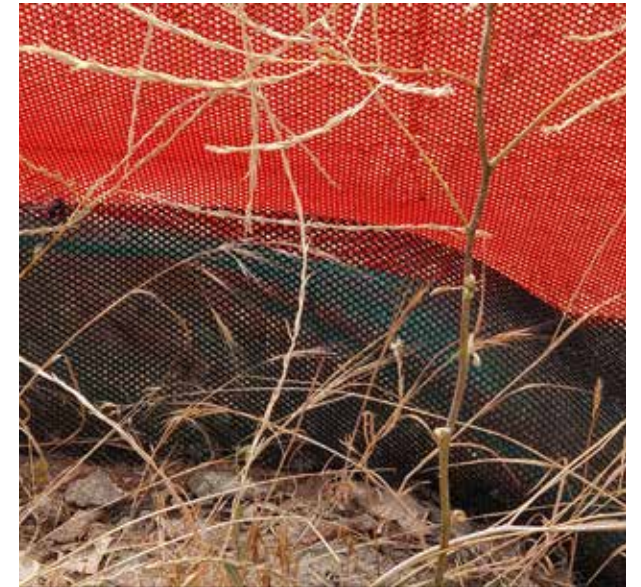
Lightweight plastic mesh with a high transparency and percentage of open area
